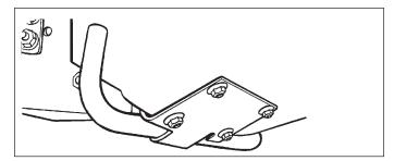
Figure 8. Engage Stone Guard Hook
